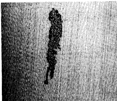
写真2 鏡面機械研磨上に生じた錆 Photo. 2 Rust on mirror-mechanical polished surface
