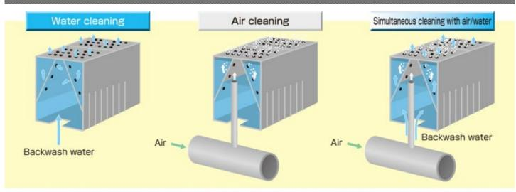
Backwash water is dispersed more evenly by pressure equalization with 2-stage structure.
