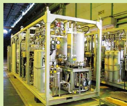
SH-20D, Special specification [simplified explosion-proof type, both H 2 and O 2 use] (6,500×2,000×2,500H)
